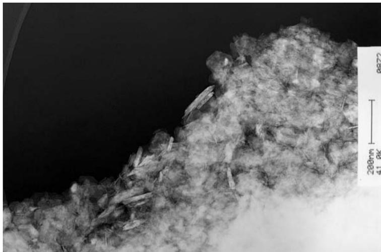
Figure 6.6: Transmission electron microscope image of synthetic  $\text{Ni}(\text{OH})_2$  from Aldrich Chemical Company. The typical grain size is  $\approx 10 - 50$  nm.
