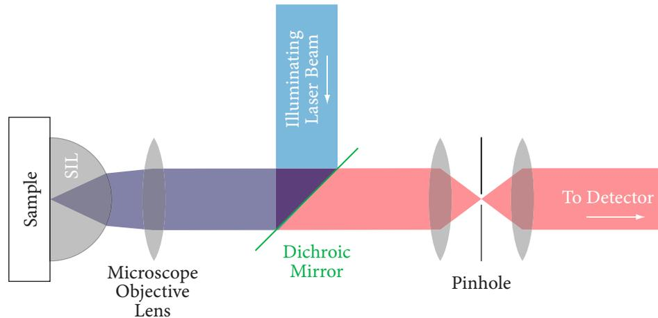
Figure 2.8: Other components to increase resolution: solid immersion lens, placed up against the sample.
