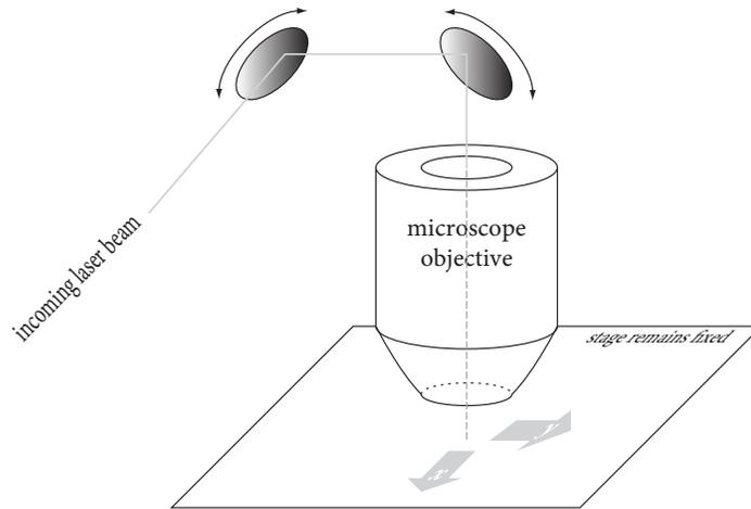
Figure 2.3: Confocal microscope instrumentation: beam scanning, with two moveable mirrors that move the beam itself.
