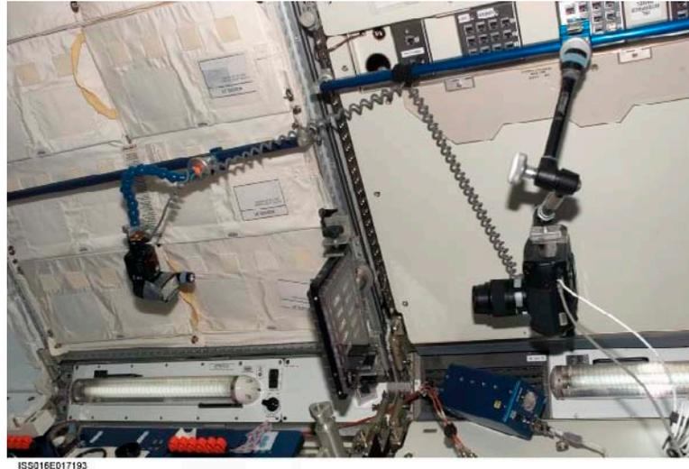
Figure 11.14: Image of the most recent EarthKAM-driven BCAT setup by Dan Tani, demonstrating a number of improvements over the MWA-based manual photography setup. The set up is clamped to the ceiling, out of the way and less prone to vibration. The illumination is now provided by a camera flash, and the camera is now tethered to, and controlled by, a laptop running the EarthKAM software.
