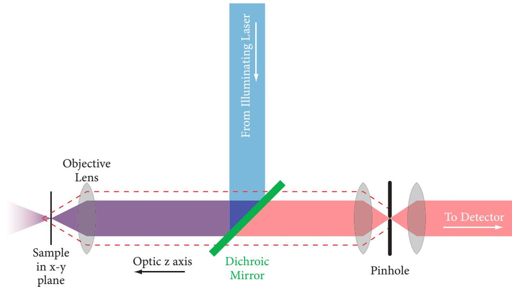
Figure 2.1: Schematic diagram of a confocal microscope. Laser light (blue) is reflected by the dichroic, and illuminates the sample at the focus of the objective. This excites fluorescence, and the sample then emits light at a lower wavelength (red), which goes through the objective, passes through the dichroic, and is focused down to a spot surrounded by a pinhole. Light from other locations in the sample goes through the objective and dichroic, but is rejected by the pinhole (red dotted line).
