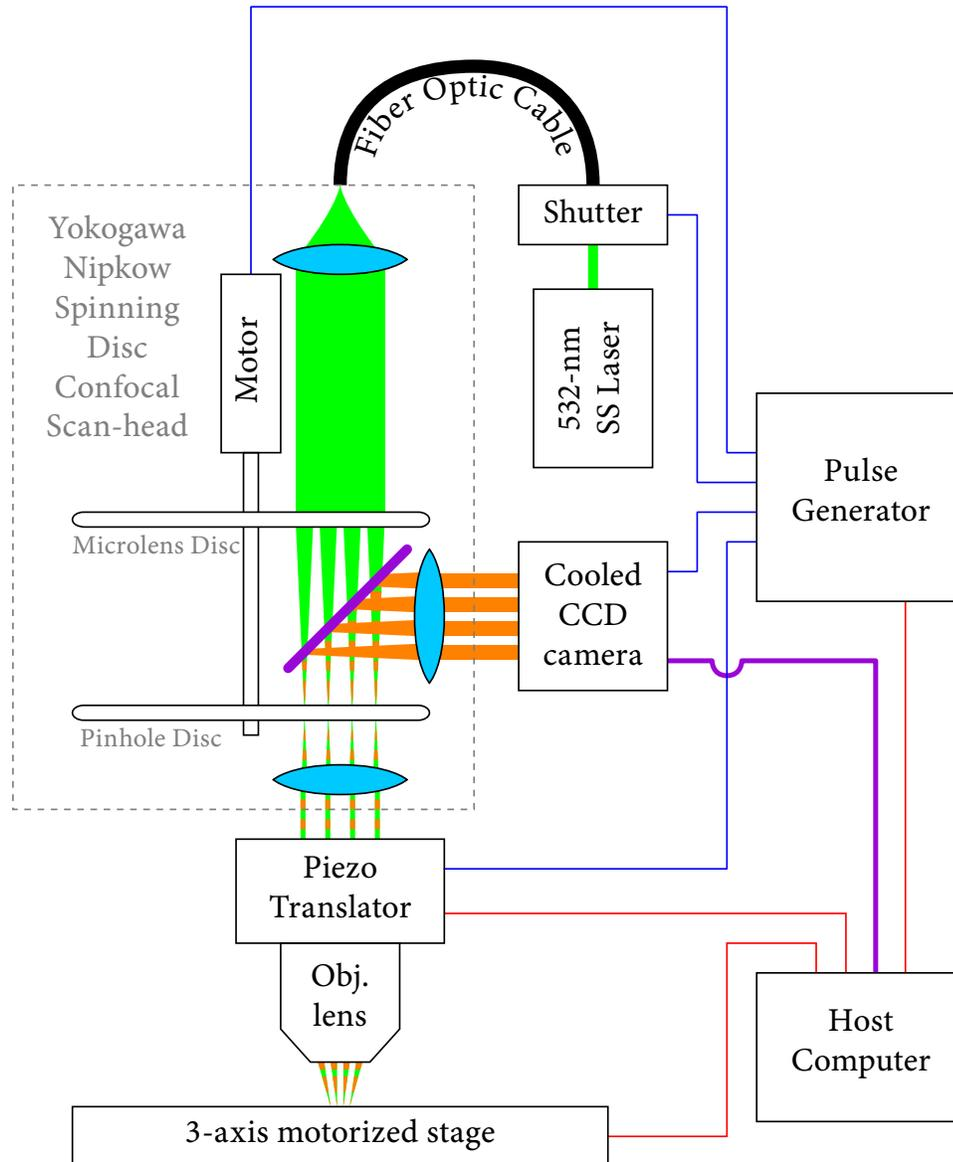
Figure 4.1: Block diagram of the TARC system (not to scale). Major components indicated by black boxes. The beam path is labeled in green (excitation) and orange (emission), with lenses in light blue. TTL signal connections are indicated with blue lines; RS-232, with red; and IEEE1394 firewire, with purple.
