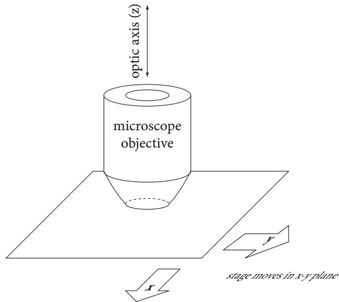
Figure 2.2: Confocal microscope instrumentation: stage-scanning, in which the optical train remains fixed and the stage is moved.
