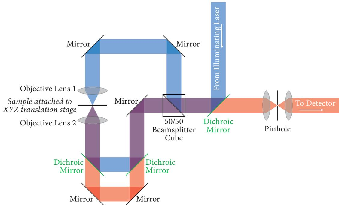
Figure 2.5: 4Pi-A configuration, with two illumination paths, but only one detection path.
