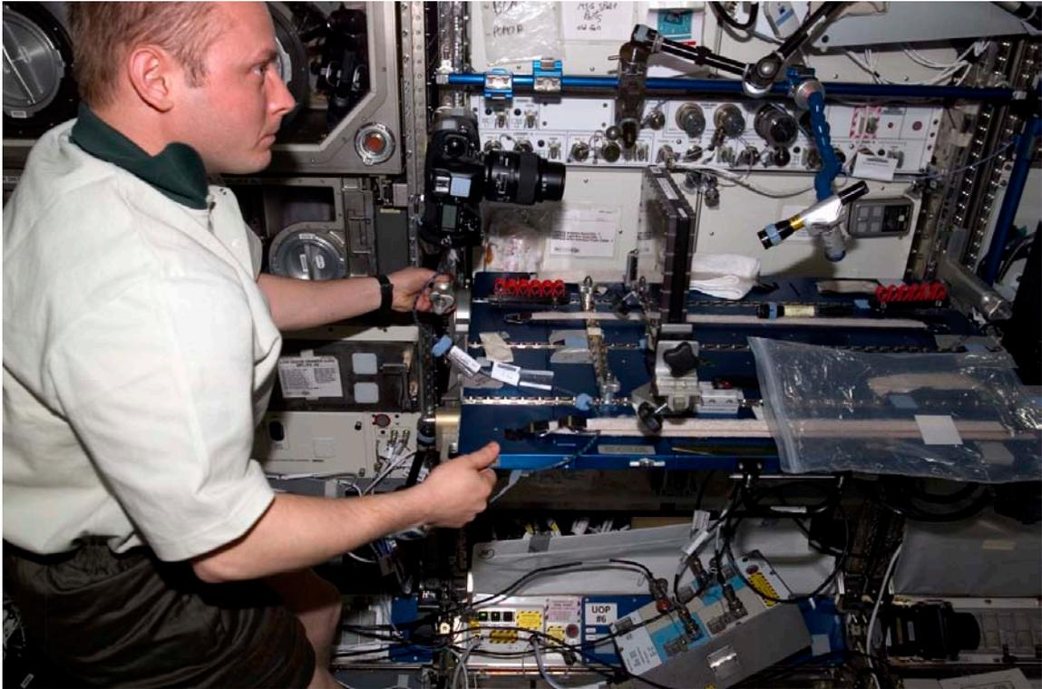
Figure 11.10: Astronaut Mike Fincke aboard the International Space Station, operating the BCAT3 experiment by taking photographs of the samples in their holder, illuminated with a flashlight from the rear.
