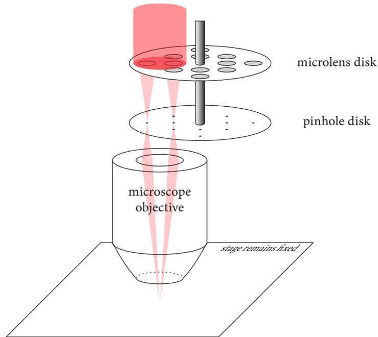
Figure 2.4: Confocal microscope instrumentation: Nipkow disk, where rotating disks of microlenses and pinholes parallelize the illumination beam.
