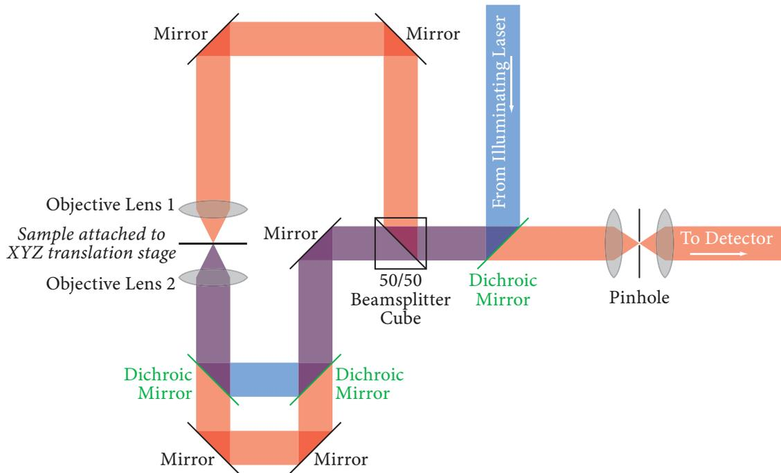
Figure 2.6: 4Pi-B configuration, with only one illumination path, but two detection paths.
