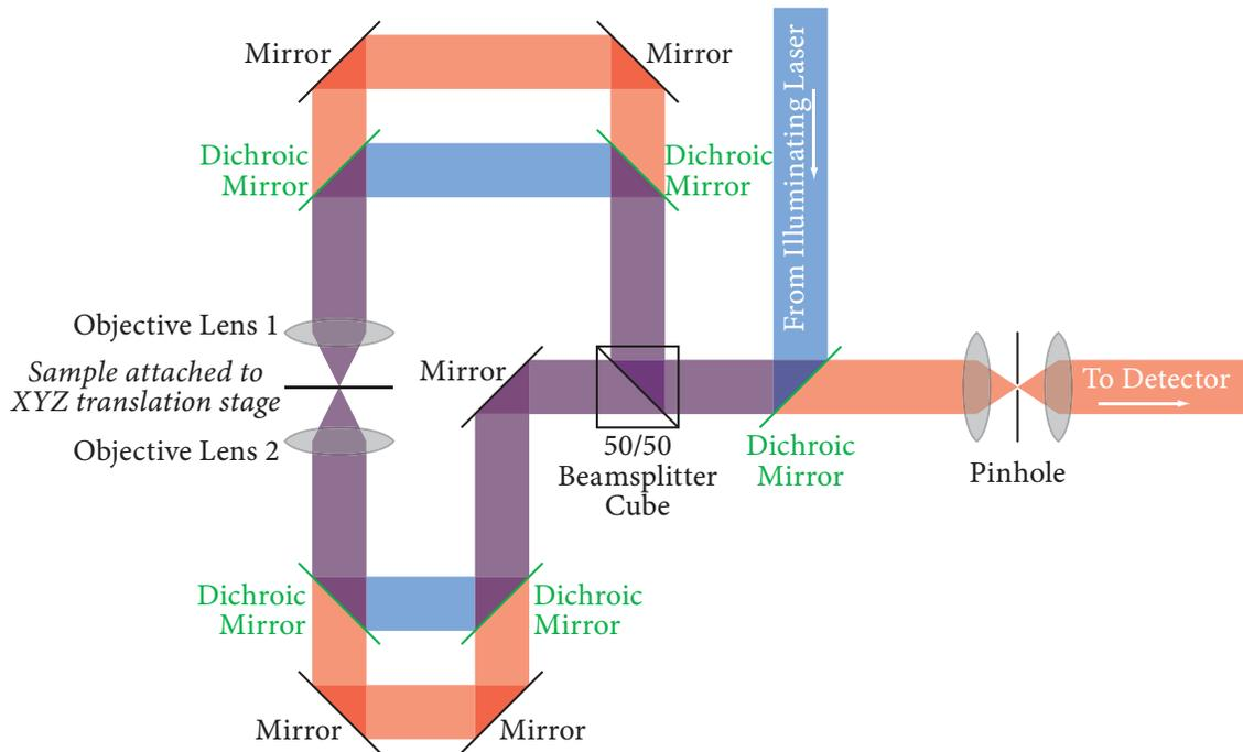
Figure 2.7: 4Pi-C configuration, with two illumination and detection paths.
