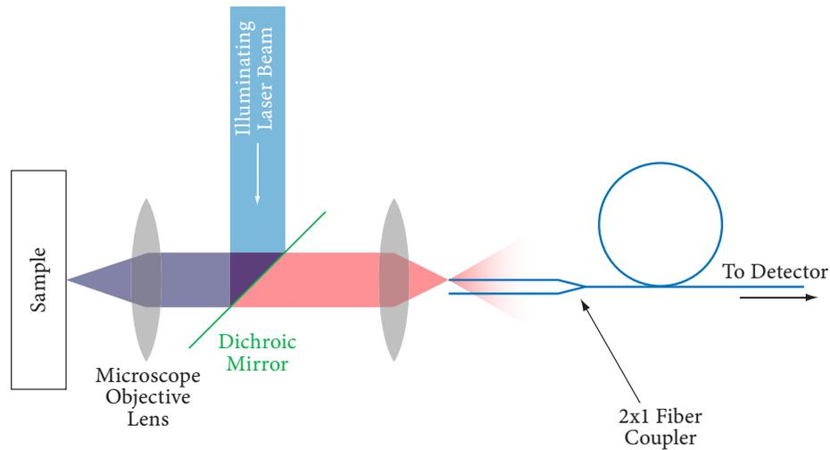
Figure 2.9: Other components to increase resolution: 2x1 optical coupler to interfere the light from the two fibers.
