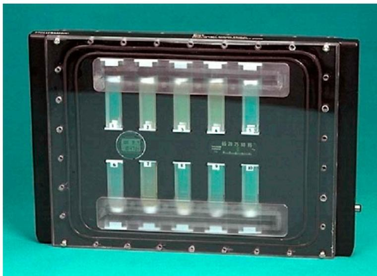
Figure 11.8: Sample holder for BCAT3 and BCAT4. Ten glass cuvettes hold all samples. The BCAT3 colloid-polymer samples described here occupy samples 1 through 6. Samples 1 through 5 fill the top row; sample 6 is the leftmost sample on the bottom row).
