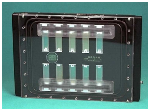
Fig. 1 BCAT sample holder with ten glass cuvettes in an anodized aluminum frame, between two sheets of plexiglass
