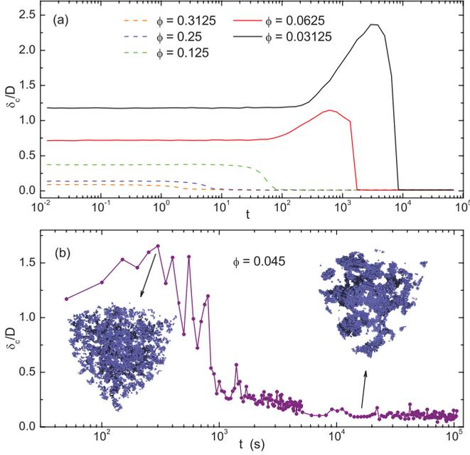
FIG. 3. (Color online) (a) Time evolution of the critical connectness distance  $\delta_c$  for gels simulated at different  $\phi$ , with  $t$  in units of  $D\sqrt{m}/u_0$ . (b) Time evolution (in seconds) of the critical distance extracted from the measured spatial positions of PMMA particles in a polymer-colloid system [7]. For times larger than about  $10^4$  s the system is in an arrested gel state.
