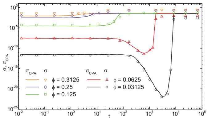
FIG. 4. (Color online) Time evolution of conductivity  $\sigma$  for  $\xi/D = 0.1$  during the formation of the colloidal gel. Numerical solution of the tunneling resistor equations shown with symbols;  $\sigma_{\text{CPA}}$  obtained from Eq. (3) using  $\sigma_0 = 0.1$ , with solid lines.
