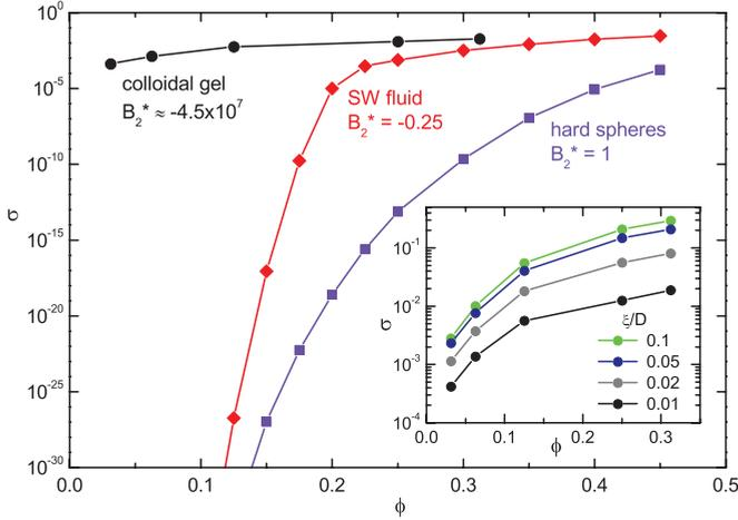
FIG. 5. (Color online) Conductivity  $\sigma$  as a function of  $\phi$  for the arrested gel state (filled circles), equilibrium SW fluids (filled diamonds), and equilibrium HS fluids (squares). In all cases,  $\xi/D = 0.01$ . Inset:  $\phi$  dependence of  $\sigma$  for the arrested gel state calculated for different values of  $\xi/D$ .
